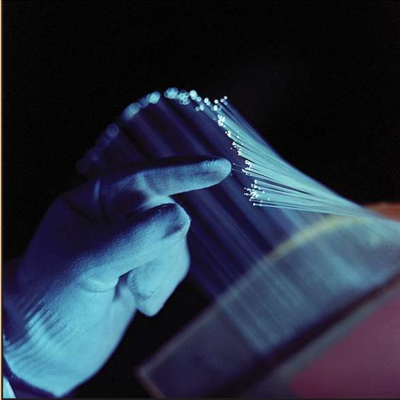
Figure 7. Photograph of lithium-doped scintillating fibers. Figure courtesy of Mary Bliss, Pacific Northwest National Laboratory.
