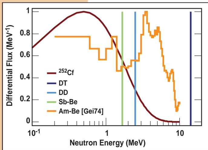
Figure 20. Comparison of normalized neutron energy spectra emitted by various nuclear reactions. Note that energies for the DD and DT reactions correspond to emissions at zero degrees.
