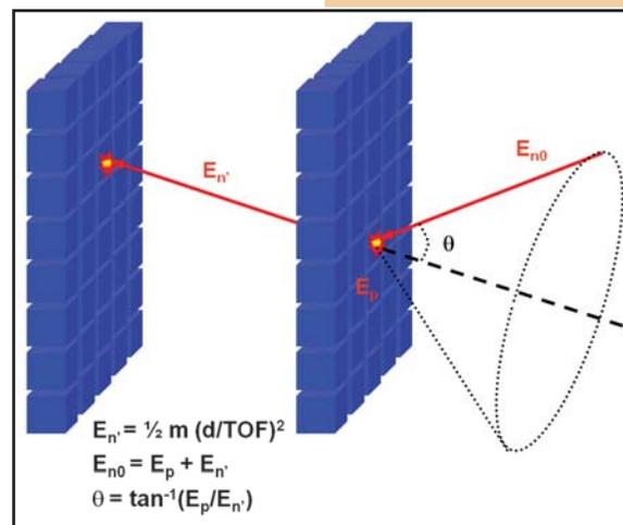
Figure 16. Diagrammatic representation of neutron scatter camera operation.  $E_{n0}$  refers to the energy of the incoming neutron, and  $E_n$  the energy of the neutron scattered from the front detector plane to the rear. Figure courtesy of Nick Mascarenhas, Sandia National Laboratories.
