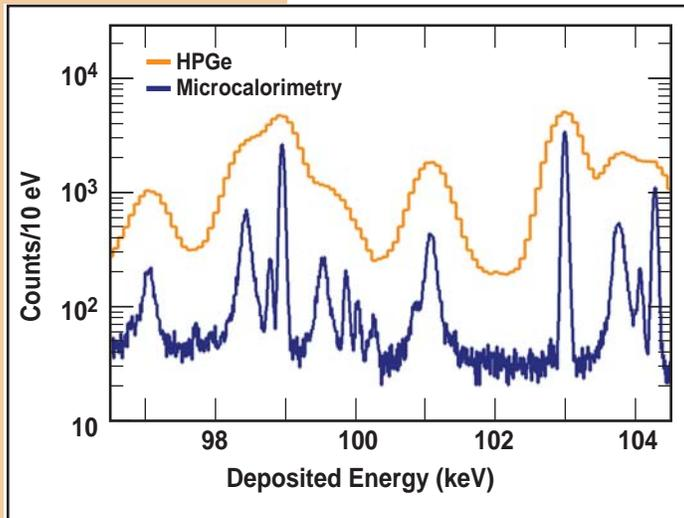
Figure 3. Plot of counts versus deposited energy acquired using microcalorimetry as compared to that of HPGe. This figure demonstrates the separation of various low-energy peaks in Pu not achievable with HPGe. Figure courtesy of Michael Rabin, Los Alamos National Laboratory.
