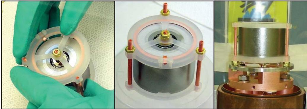
Figure 2. Photographs of high-purity germanium crystal assembly including insulator (clear plastic), high-voltage contacts (copper ring and center wire), and cold plate (bottom of right-hand photograph). Figure courtesy of Jim Fast, Pacific Northwest National Laboratory.
